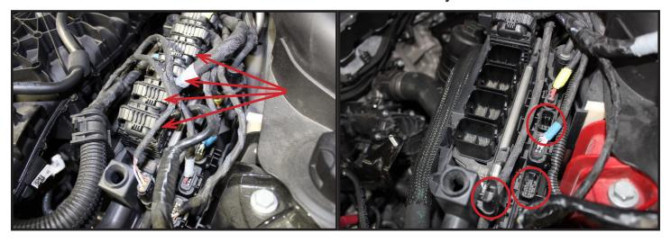
5. With everything on top of the manifold out of the way, disconnect the water lines underneath the manifold. Use a small pick tool to pop the retaining clip out and remove the hose from the fitting.
