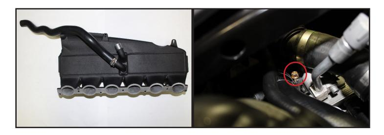
12. Inspect the included gasket for any damage and install it on the flange of the cylinder head. To help keep the gasket in place while installing the manifold, use a thin layer of copper gasket maker and allow it to get tacky before proceeding.
