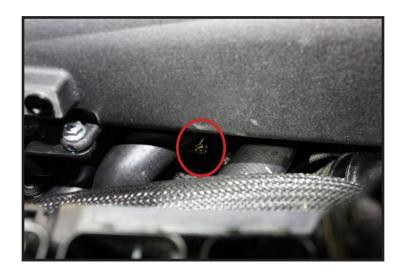
18. With the manifold in place, now assemble your fuel vapor feed hoses. Using the existing hoses cut off the hoses with a razorblade by carefully cutting a small incision where the hose meets the connector (pictured above), make sure not to cut too deep as you will damage the connector.
